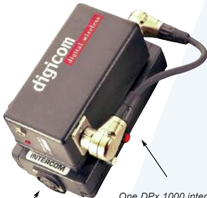
Wired system connects here
