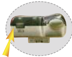
"Talk" BUTTON adjusts to either transmit or listen-only mode.
